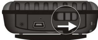
**| CAUTION:** Always leave the ON/OFF switch in the ON position for normal operation.
